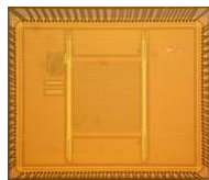
32 x 32 time-resolved optical detector
